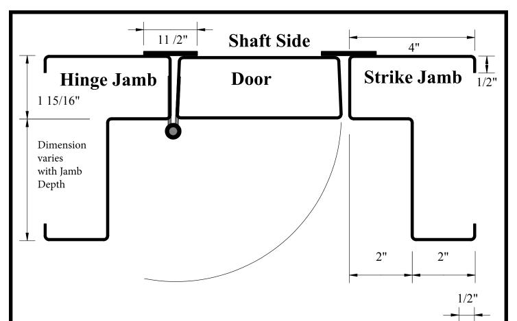
Smallest jamb depth available for a HC elevator shaft frame is 3 1/2" (2 1/2" Wall Dimension).
