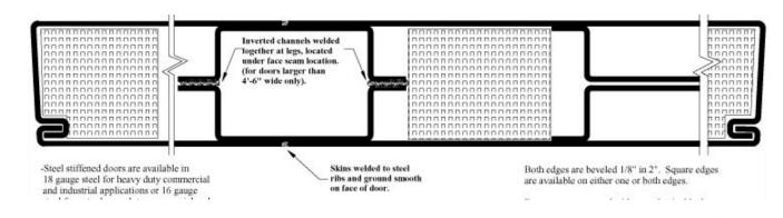
Oversized Steel Stiffened Doors are for doors 5'0" x 10'2" single opening size
